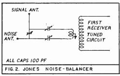
If you don't want to dig into the innards of your rig, this circuit should also work with its center-tapped coil positioned around the tuning coil in your antenna tuner, if you happen to use one. Experimenting with the number of turns and coil placement is likely to improve performance of the circuit. One note of encouragement: patience and perseverance are said to be essential when working with noise-balancing circuits.
